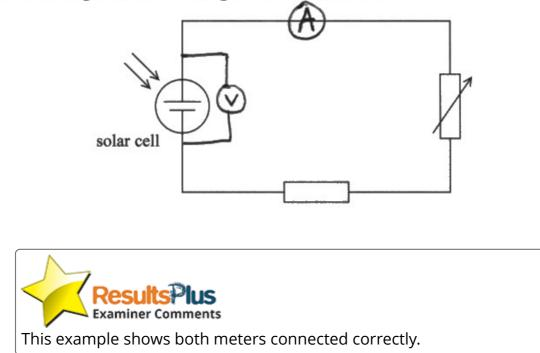
(b) The student investigated how the potential difference across the solar cell varied with the current through the solar cell.
